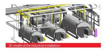
After that the creation of the model was done in Autodesk Revit software, involving information of steam boilers, piping, insulation and mechanical equipment.
