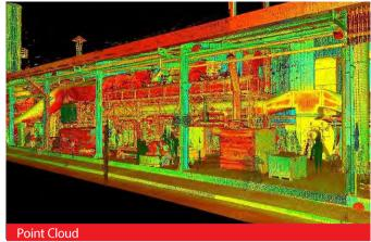
The first action was to place an adequate number of black and white targets all around the installation. These marks were well recognizable, and they had the size of an A4 paper. Additionally, our team used four smaller targets to offer additional constraints capturing their position with the use of the highest accuracy industrial total station Leica TDRA6000. The installation was covered through 75 laser scanner setup positions with over 2 billion points.
