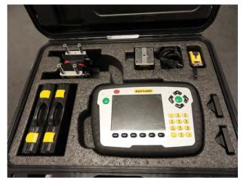
Easy Laser E 710 Shaft Alignment System
