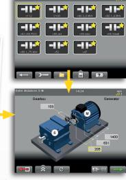
Using the barcode reader, you scan the appropriate tag and the correct measures for that specific machine are entered automatically. Or open the settings with the pre-defined machine templates. Quick and easy! Included with Vestas 3 and 4.
