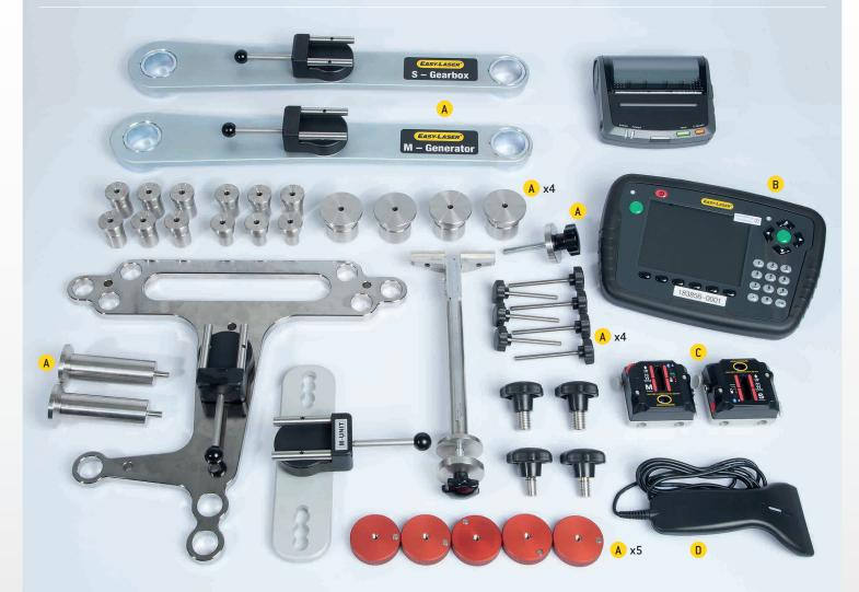
System Easy-Laser® Vestas 4 A. V112 brackets and accessories B. E52 Display unit C. Measuring units ELS40 and ELM40.
